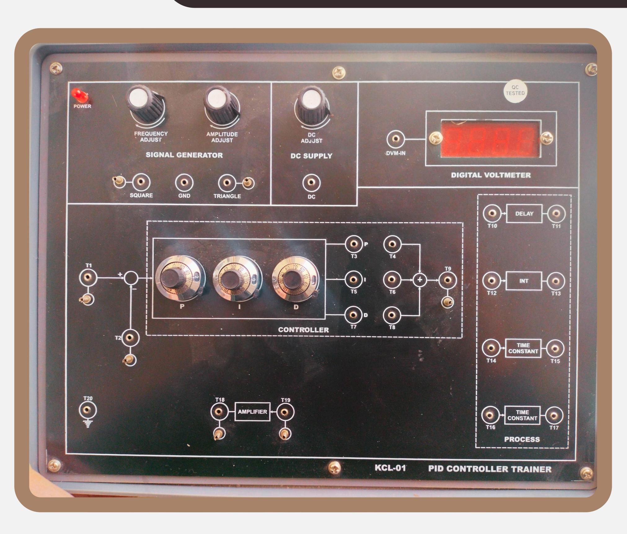
scenarios and master the intricacies of control systems. Developed specifically for PID Controller enthusiasts, this trainer offers hands-on experience in tuning and optimizing PID parameters. . Unlock the potential of PID control with the P, PI, PID Controller Simulator Trainer (KCL-01), an invaluable tool for
