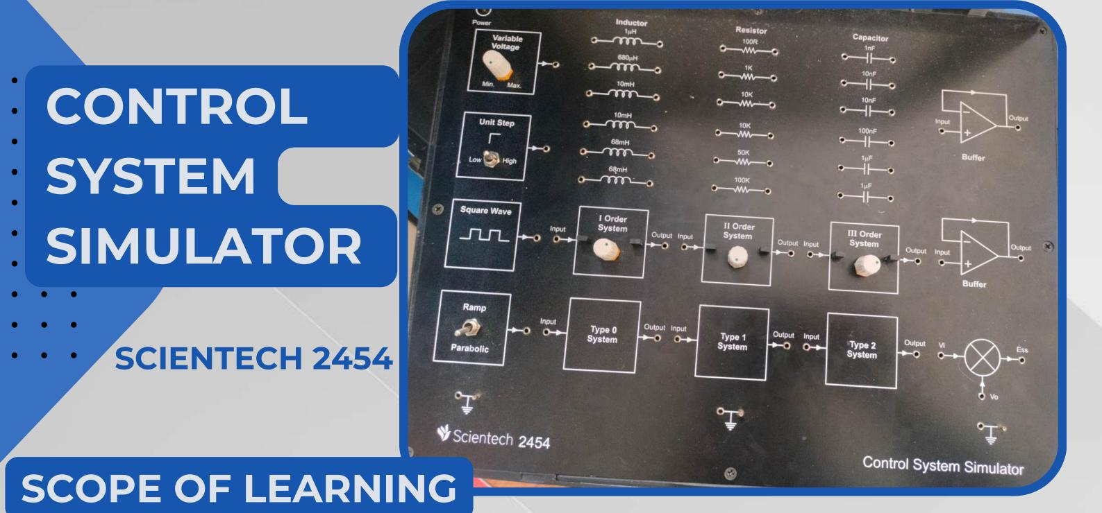
To observe the First Order control system for different values of the Damping Ratio at different values of resistance To observe the Second Order control system for different values of the Damping Ratio at different values of resistance To observe the Third Order control system for different values of the Damping Ratio at different values of resistance To observe the Type0 control system Steady State Error (Ess) for Unit Step or Square wave input
